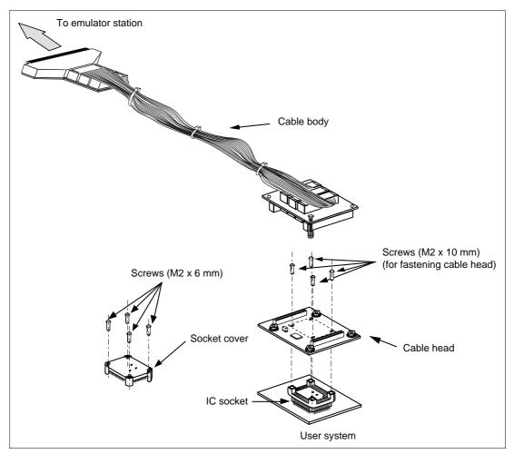
Figure 1 HS2338ECH61H User System Interface Cable
